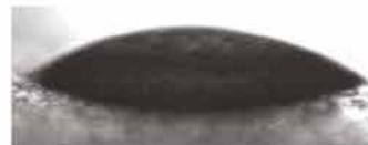
MOULEX® WD401 wettability on a mold surface WITH BOUCHEX
